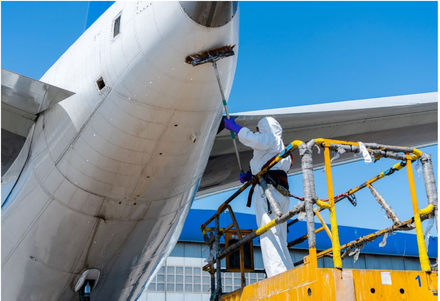
Regular deep washing is key to prevent corrosion
