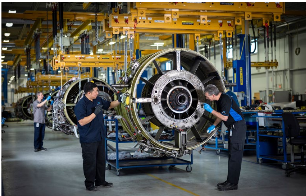
CFM56-7B case inspection
