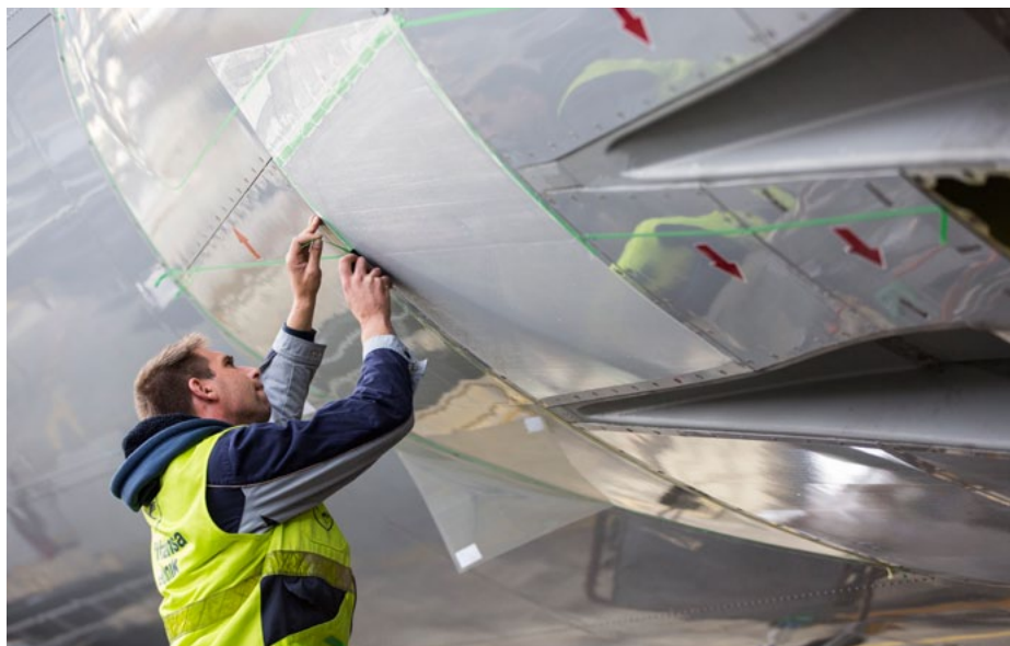
Drag-reducing film AeroSHARK
