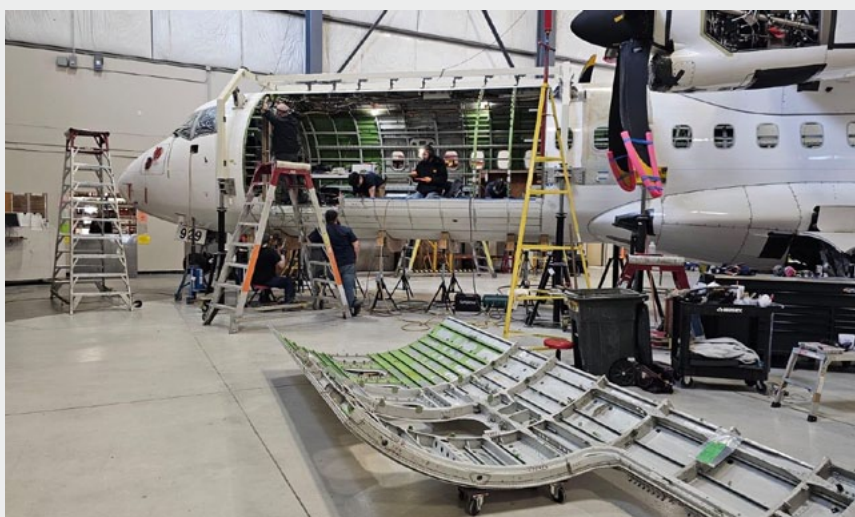
Work in progress of the conversion of a new large cargo door (LCD)
