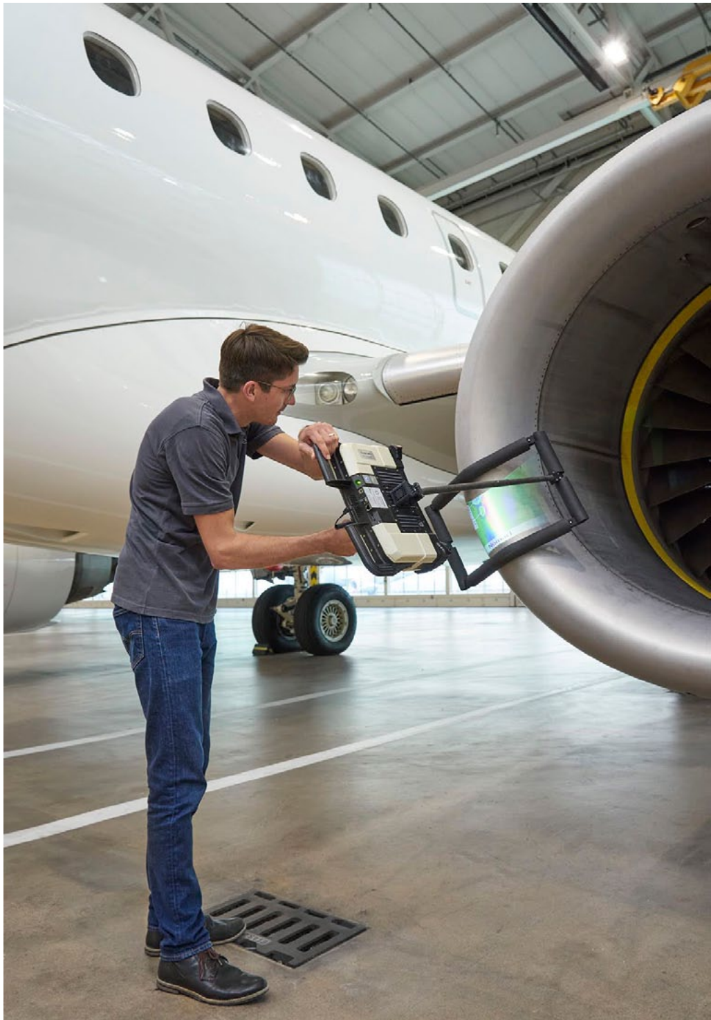
Performing a leading-edge scan with the dentCHECK tool
