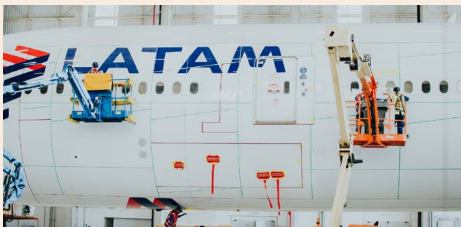
The AeroSHARK surface film is applied to a LATAM aircraft
