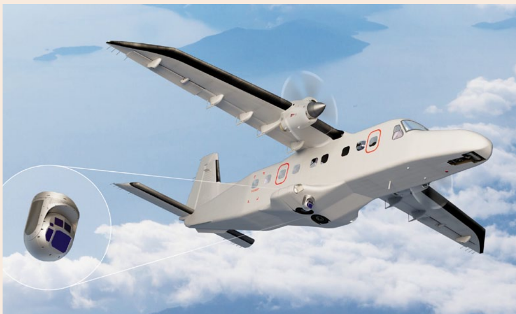
The TrakkaCam is a multispectral imaging system designed for surveillance and reconnaissance missions
