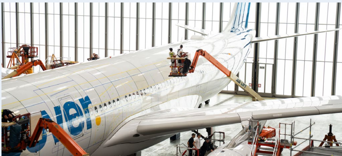
Applying AeroSHARK 'shark skin' on the A330 aircraft
