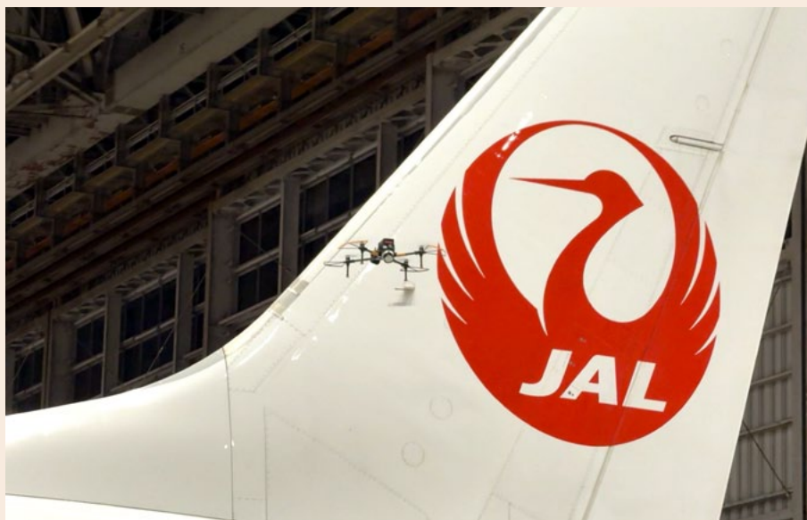
Drones capture high-resolution images of aircraft exteriors for mechanics to review
