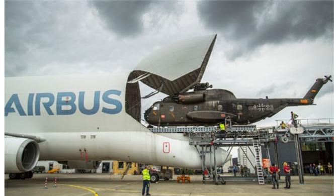
Lifting of a CH53 military medium-lift helicopter into the Beluga Photo: Airbus
