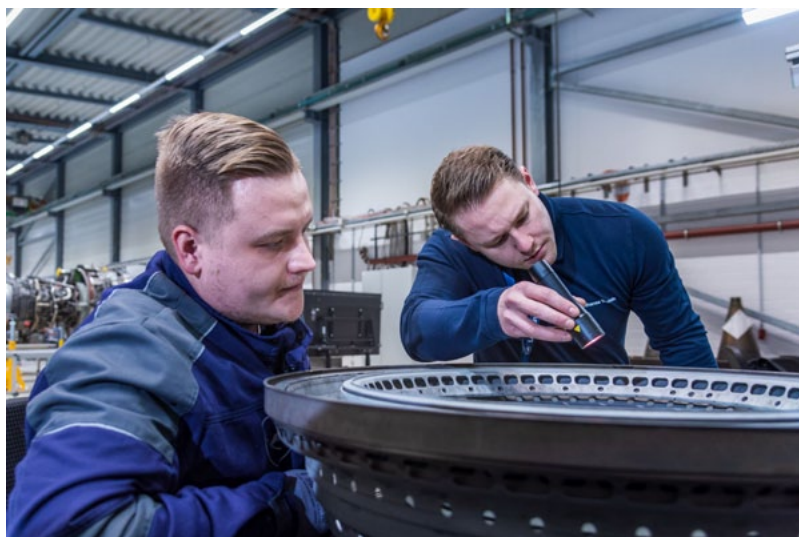
Mechanics inspecting a combustion chamber
