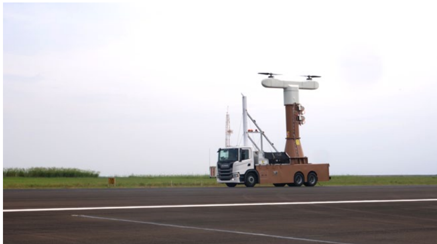
Eve Air Mobility began testing its vertical lift rotors aboard a new custom truck-mounted platform
