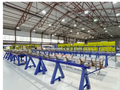
New manufacturing jigs are in place at Britten-Norman's Bembridge facility in preparation for production output increase © Britten-Norman
