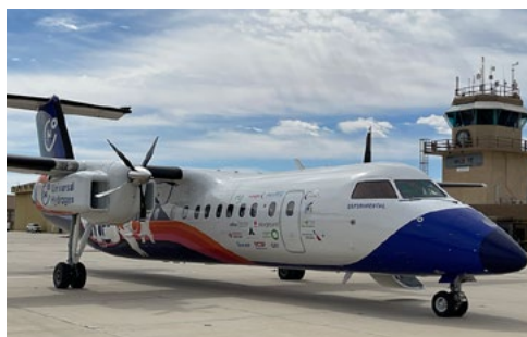
Dash-8 modified 40-passenger regional airliner, powered on one side by a hydrogen fuel cell powertrain © Universal Hydrogen
