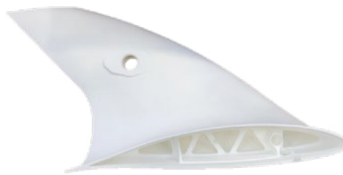
Additively manufactured wingtip for Eviation's Alice, the all-electric aircraft © Materialise
