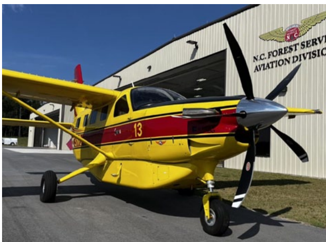
Daher's first Kodiak 100 delivered with a five-blade composite propeller is shown at the North Carolina Forest Service's Aviation Division © Daher
