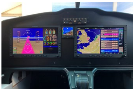
VoltAero's Cassio 330 full-scale cabin mock-up includes a flight deck equipped with Avidyne's Quantum 14-inch displays in the dual PFD/MFD configuration © VoltAero
