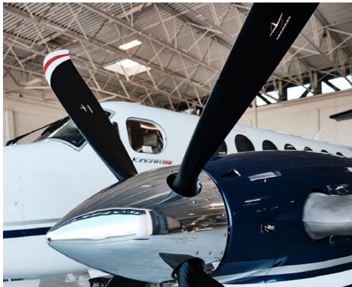
McCauley's newest C780 propeller for the Beechcraft King Air B300 series © Textron Aviation
