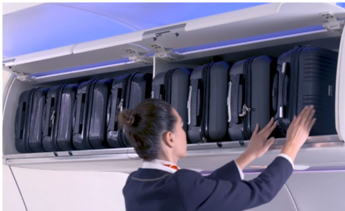
The Airspace L Bins will provide a 60% increase in cabin luggage storage space © Lufthansa
