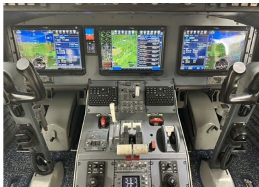
West Star Aviation CHA has successfully installed a Collins Pro Line Fusion® integrated avionics system in a Challenger 604 jet © West Star Aviation
