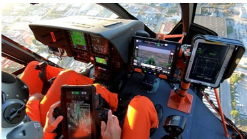
Airbus Helicopters' FlightLab flew fully automated from lift-off, taxi, take-off, cruise, approach and landing © Airbus
