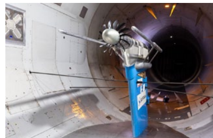
© Safran and ONERA have started wind tunnel tests with ECOENGINe, a 1:5 scale demonstrator of the forthcoming Open Fan technology
