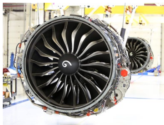
New LEAP-1B engines being prepared to ship to Boeing for the 737 MAX from facility in Peebles, Ohio © CFM International
