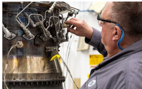
A Pratt & Whitney engineer inspects a full annular combustor rig at the company's test facility in Middletown, CT © Pratt & Whitney
