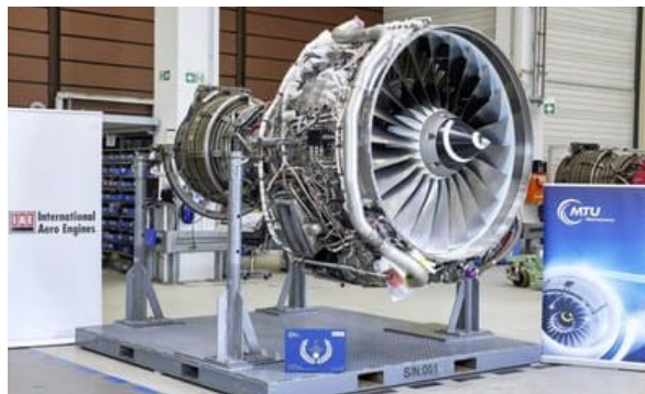
IAE has tested the V2500 engine with 100% SAF at MTU Maintenance Hannover, Germany © Pratt & Whitney
