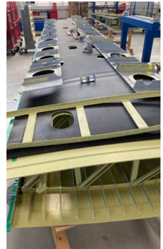
Final assembly of Do228 NXT wing © GA-ATS
