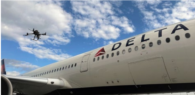
Delta is using drones for visual inspections of its aircraft © Delta TechOps
