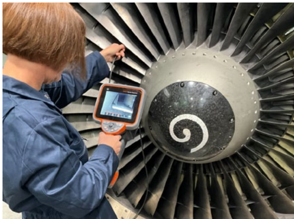
An inspection is being conducted using Waygate Technologies' Mentor Visual iQ+ borescope © GE Aerospace
