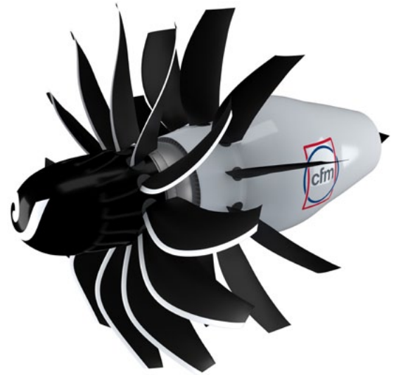
CFM Open Fan engine design
