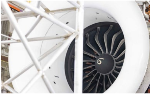
CFM has used a propriety dust ingestion rig to replicate what operators are experiencing in service © CFM International
