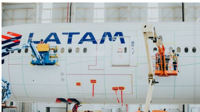
The AeroSHARK surface film is applied to a LATAM aircraft
