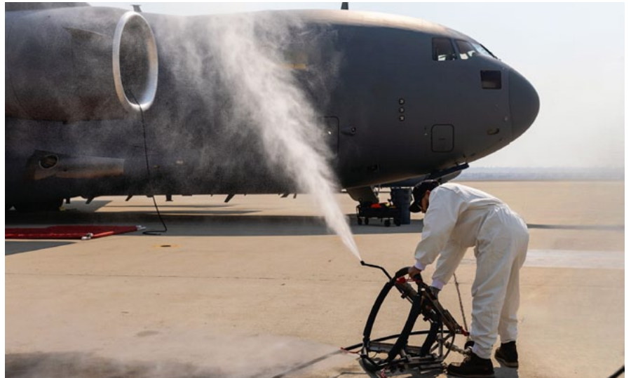
Cyclean engine wash
