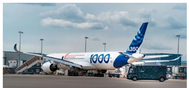
Various sensor technologies, including multiple Aeva 4D LiDAR units, are being tested on an Airbus A350-1000 flight test aircraft and an electric truck during hundreds of hours of taxi operations © Airbus UpNext
