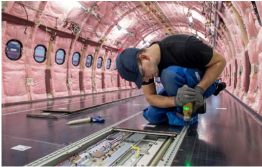
Station 41, A320 family final assembly line installation floor panels © Satair
