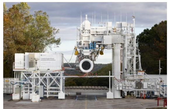
GE Aerospace has made the first ground test of a commercial hybrid electric engine demonstrator
