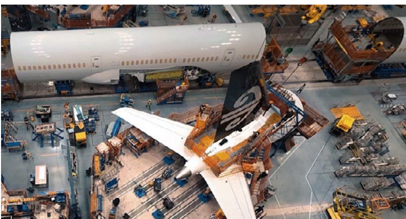
Sections of the enhanced 787-9 are loaded into final assembly
