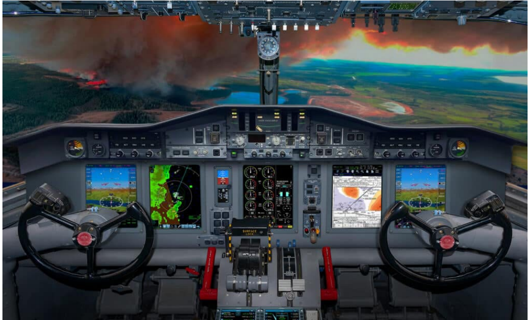
The InSight Flight Display System has received STC approval for the DHC CL-415 amphibious firefighting aircraft © De Havilland Canada
