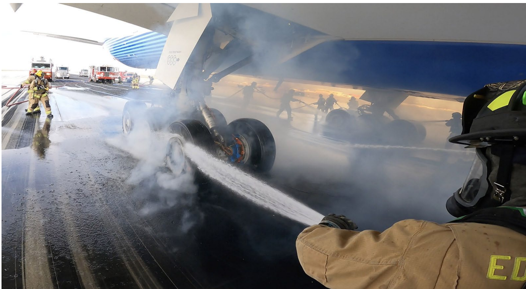
Crews respond to cool the brakes and wheels after a five-minute waiting period had passed
