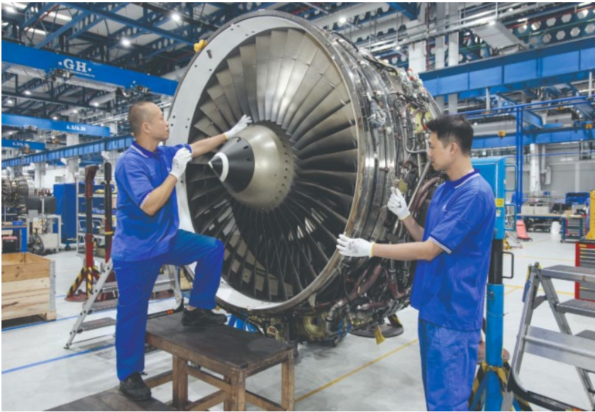
CFM56-5B engine maintenance in Zhuhai
