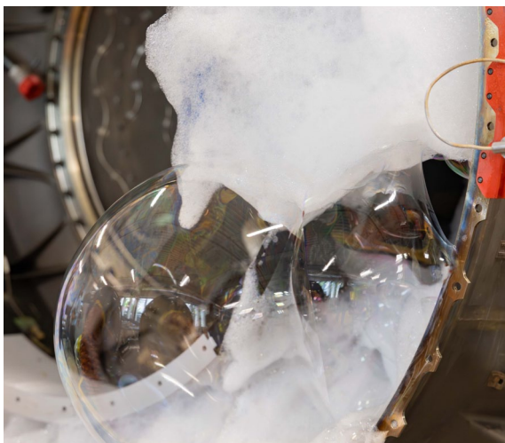
360 Foam Wash jet engine cleaning technology is being deployed to MRO shops globally © GE Aerospace
