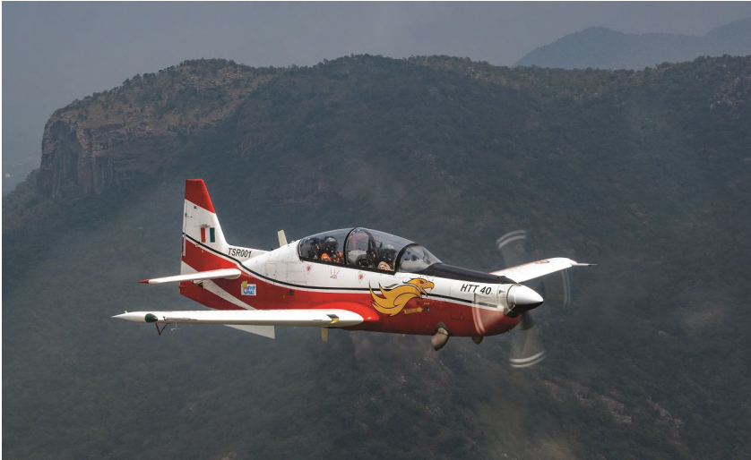
The HTT-40 basic trainer aircraft is powered by a TPE331-12B turboprop engine
