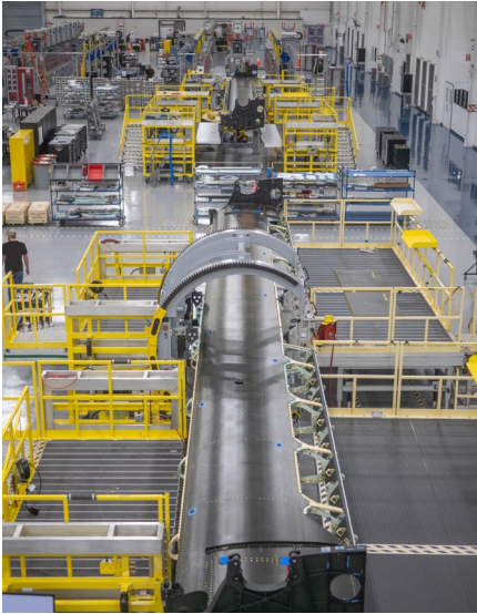
Bell has completed the first two wing structures for the MV-75 Cheyenne © Bell Textron
