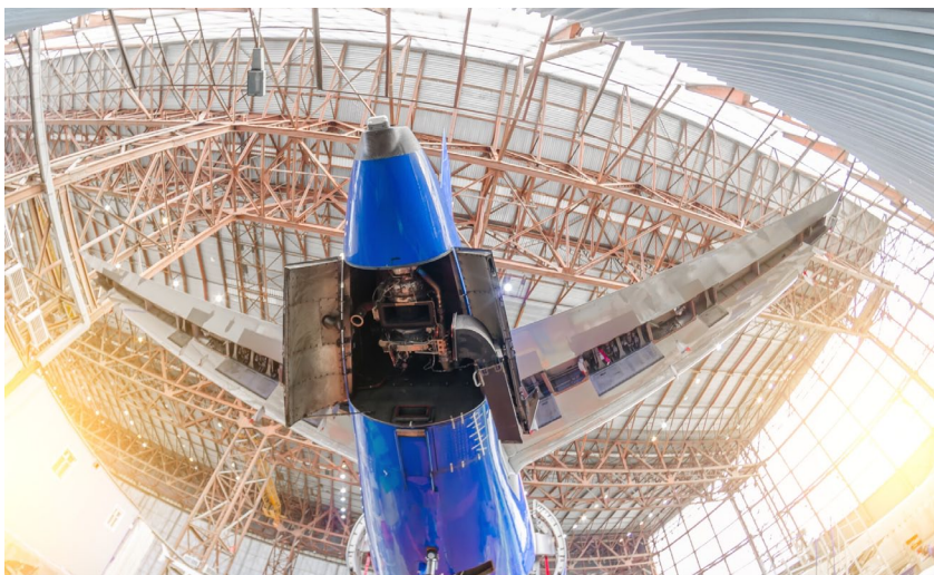
The rear section of a commercial aircraft with the Auxiliary Power Unit (APU) access doors open to expose the APU © AdobeStock
