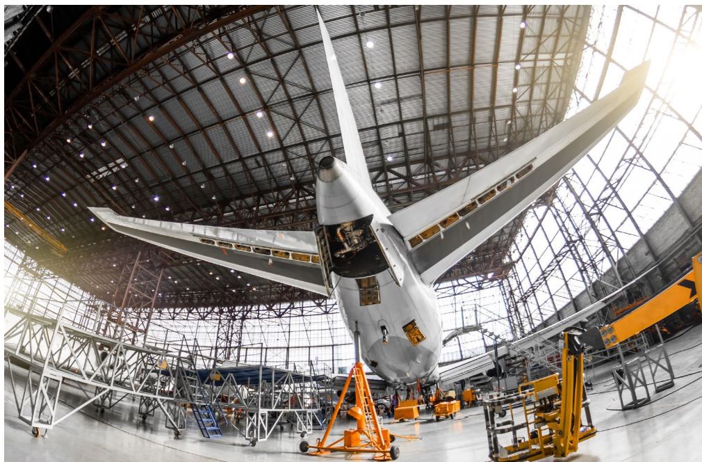
Work being carried out on an aircraft auxiliary power unit
