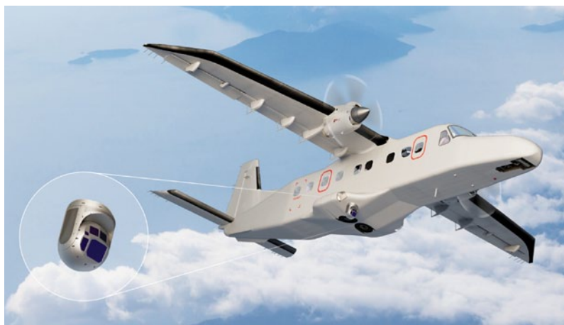
The TrakkaCam is a multispectral imaging system designed for surveillance and reconnaissance missions © GA-ATS
