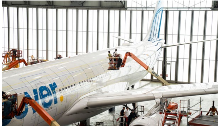
Applying AeroSHARK ‘shark skin’ on the A330 aircraft
