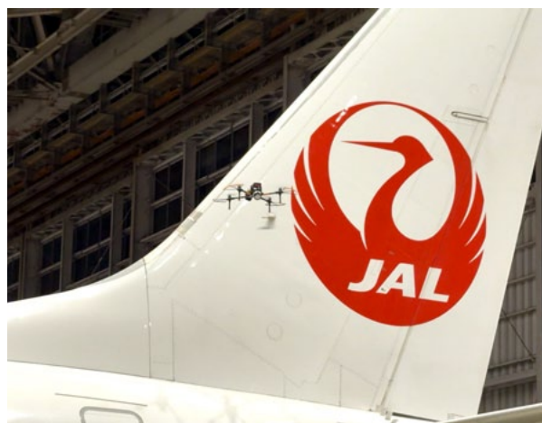
Drones capture high-resolution images of aircraft exteriors for mechanics to review © JAL
