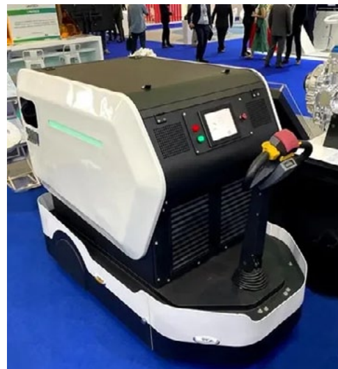
The intelligent mobile charger for Cassio airplanes and other e-aircraft © VoltAero
