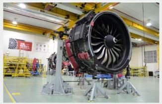
CFM LEAP-1B engine at ST Engineering's engine MRO facility in Singapore © ST Engineering
